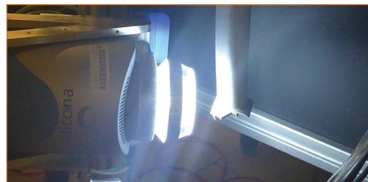
Alicon傳感器獲取點蝕的三維模型 Alicon sensor captures the 3D model of pitting
