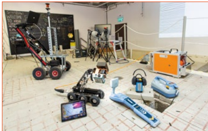
Advanced instrumentation for detecting problems of underground utilities such as leaks and voids
