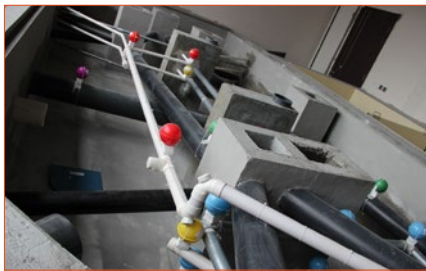
Underground utility networks in PolyU's Underground Utility Survey Laboratory
