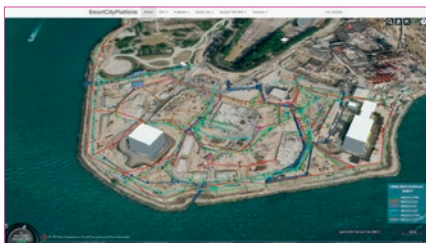
3D spatial information of underground utilities shown on the Smart City Platform
