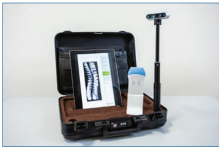
Scolioscan Air, a portable 3D ultrasound imaging system for scoliosis assessment
