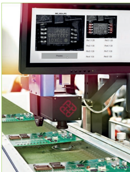
PolyU's light field sensor can be used in automated quality control, e.g. performing precision measurement on products such as semi-conductors in production lines.
