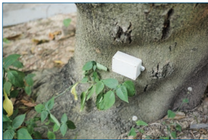
The smart monitoring system for urban tree management uses wireless sensors attached to lower tree trunks.
