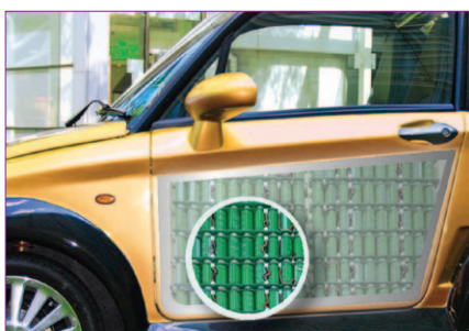
The newly developed supercapacitor module is slim enough to be fitted in almost any part of the auto body.
