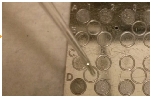
Direct oil sample loading
