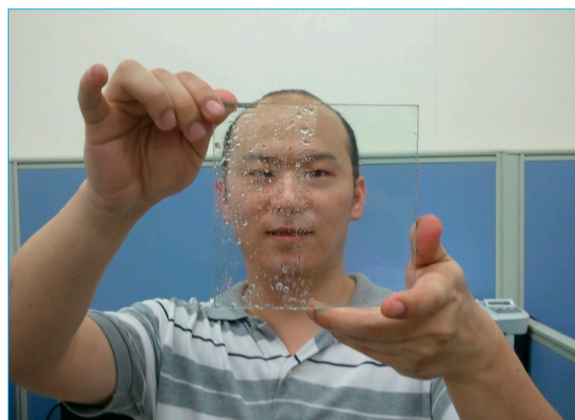
採用所研發漿料製備的自潔玻璃 The self-cleaning glass fabricated by the nanocomposite paste
