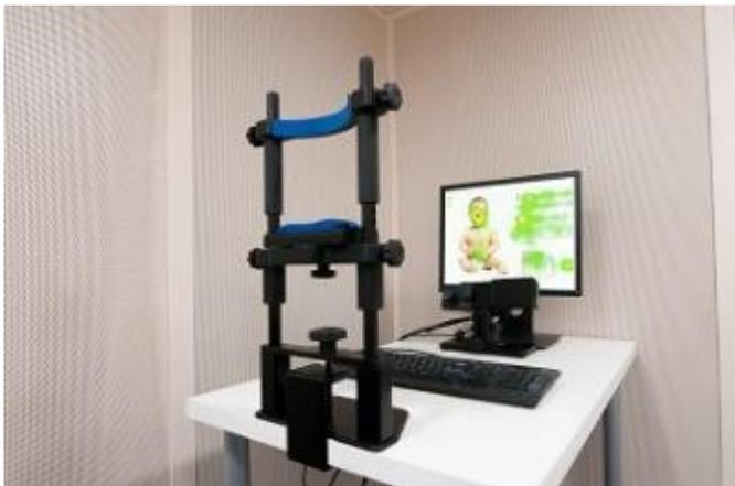
*Tobii TX300 eye tracker*, which enables unobtrusive recording of natural behaviour, is used for data collection.
