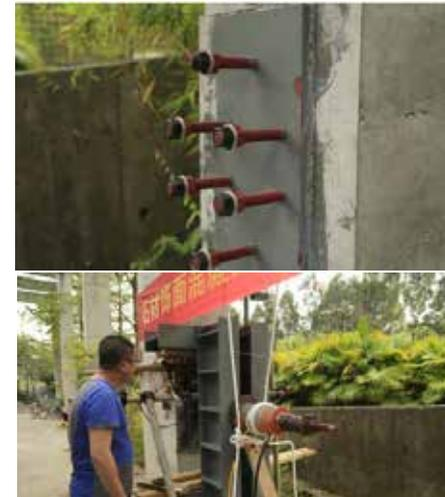
Fig.3 In-situ pull-off tests of the new stone façade system
