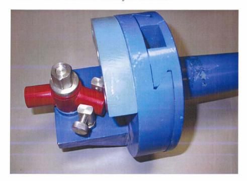
Fixture II: fixture used in milling machine
