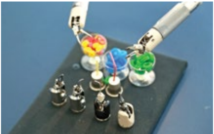
Robotic arms that reassemble inside human body to assist surgeons in single-incision or incision-less surgery 可在人體內重組以輔助外科醫生進行單切口或無切口手術的機械臂
