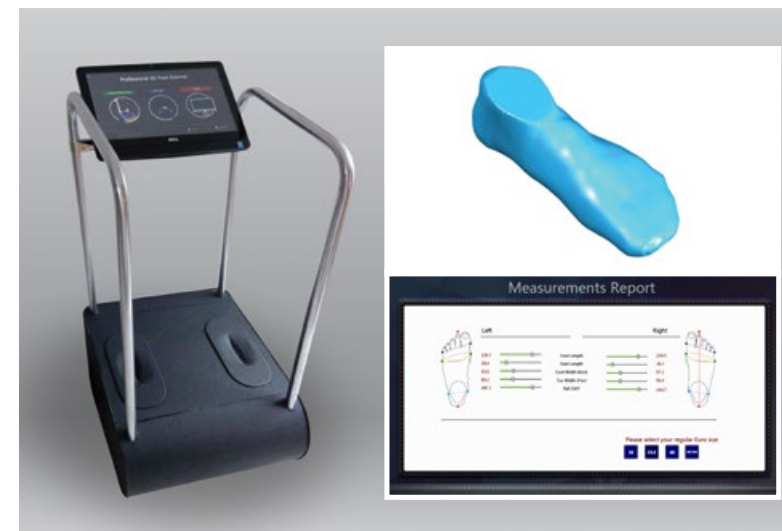
3D foot scanner and its measurement display 三維足部掃描儀及其計算結果顯示版面
