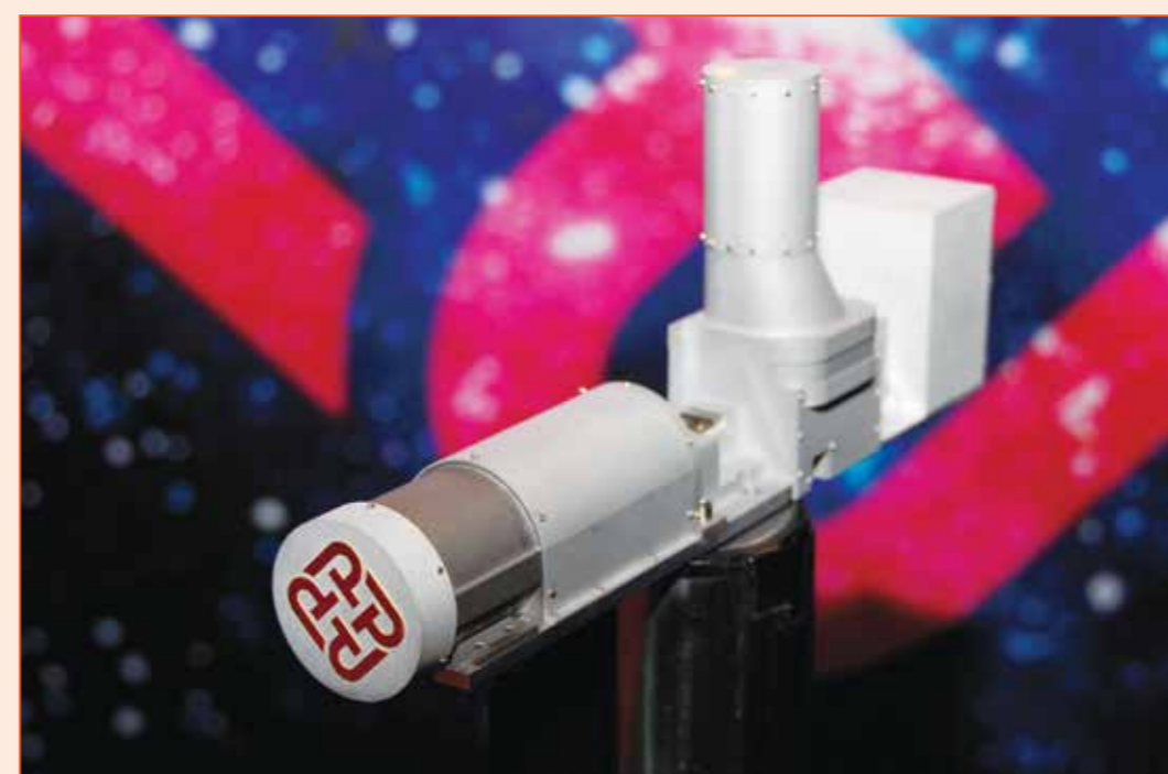
The soil preparation system for grinding and sifting Phobos rocks 用作土壤磨碎及篩選的行星表土準備系統
