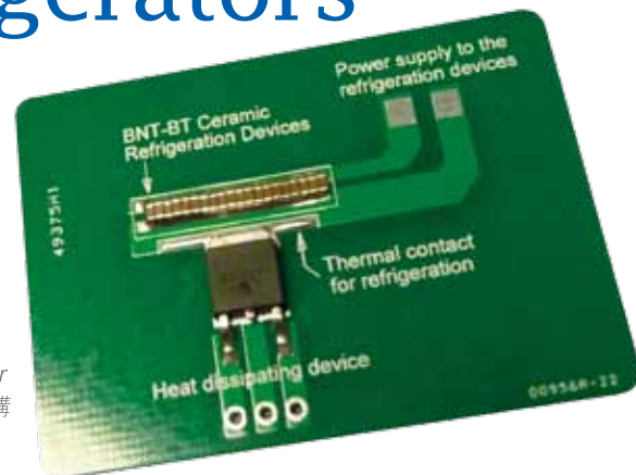
Structure of the ferroelectric microrefrigerator 鐵電微型製冷器的結構
