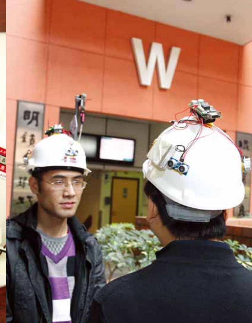
The PCMS involves the installation of GPS sensors onto the helmets of construction workers.
