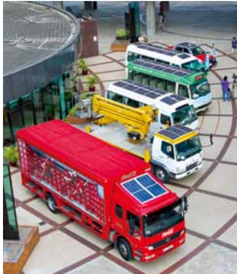
The system has been installed on different types of vehicles, including minibuses, taxis, public light buses and trucks.
