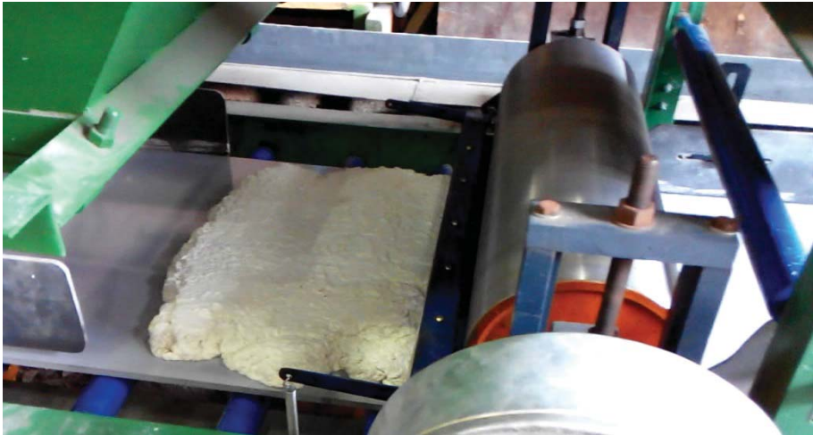
Figure 2 Glass mortar produced from the laboratory molding process
