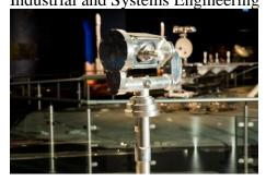
Installed on top of the lunar lander, it facilitates panoramic image capturing and rover movement observation on the moon, and helps construct a precision 3D model of the landscape for safe rovering. With a complex design and a weight of only 2.8 kg, it is sturdy enough to protect the camera against shock and vibration during the space mission and ensure its proper functioning under the extreme lunar environment.
