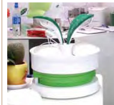
Aqualeaf: a device to automatically supply plants with water by drawing moisture out of the air. 水凝葉：可利用空氣中的水氣自動為植物提供水分。
