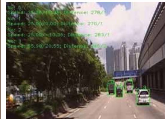
Vehicle detection and tracking by probe vehicle 利用浮動車進行車輛探測與跟蹤
