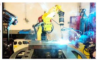
Robotic welding system at CNERC
