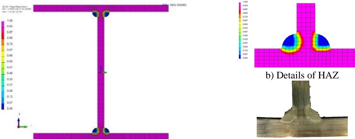
a) Predicted results after phase change and recrystallization and c) Observed HAZ after etching
