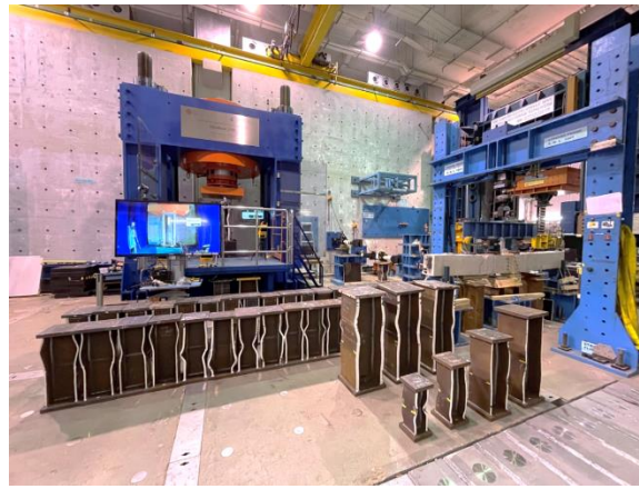
Compression tests on stocky columns of high strength S690 and S960 steel with welded splices
