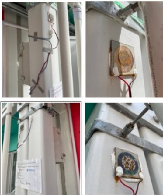
Corrosion rates monitoring in both external and internal structural steelwork of Nam cheong street modular social housing project
