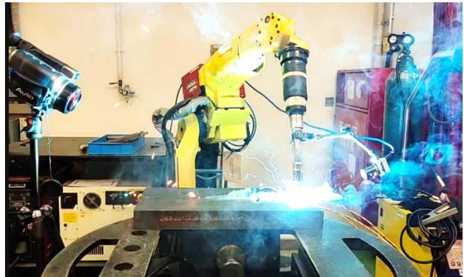
Robotic welding system at CNERC
