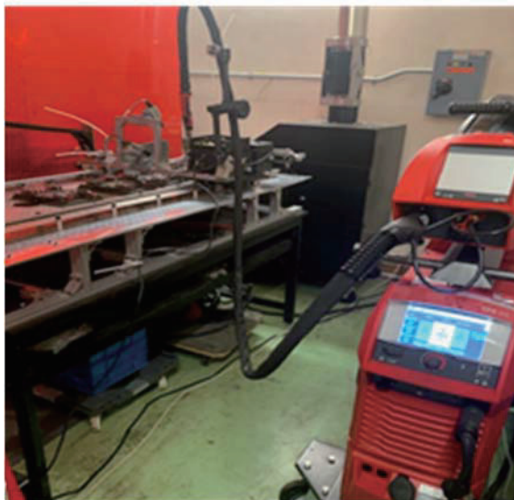
Figure 1. Automated MIG welding manufacturing system.
