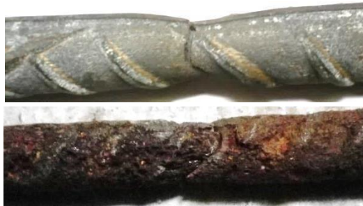
Fig. 3 Comparison of the failure point for corroded and non-corroded bars
