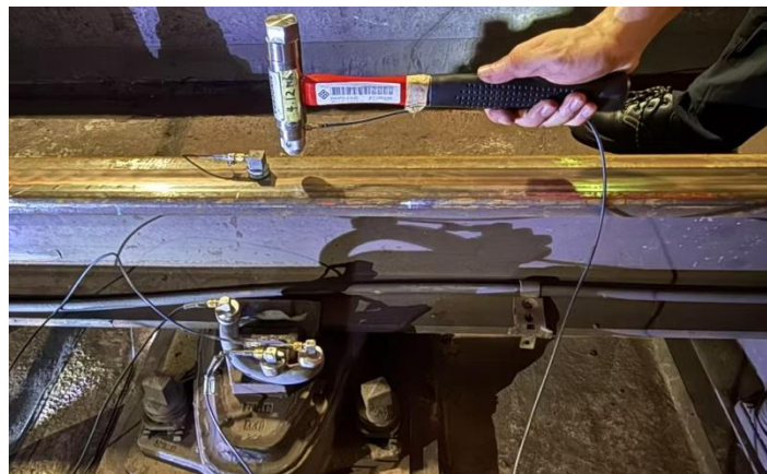
Fig 2.53 Field processing situation of the impact hammer test.
