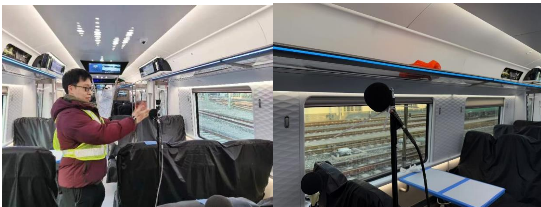
Fig 2.116 Layout of microphone sensors inside the train cabin
