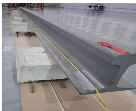
Fig 2.60 Experimental setup for railway track monitoring, (a) the DAS interrogator, (b) the rail tracks, (c) the optical fiber installed on the track and (d) the hammer to generate vibrations in the track
