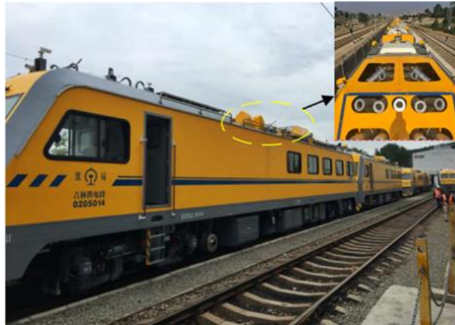
Fig 2.62 Image acquisition system of the catenary inspection vehicle
