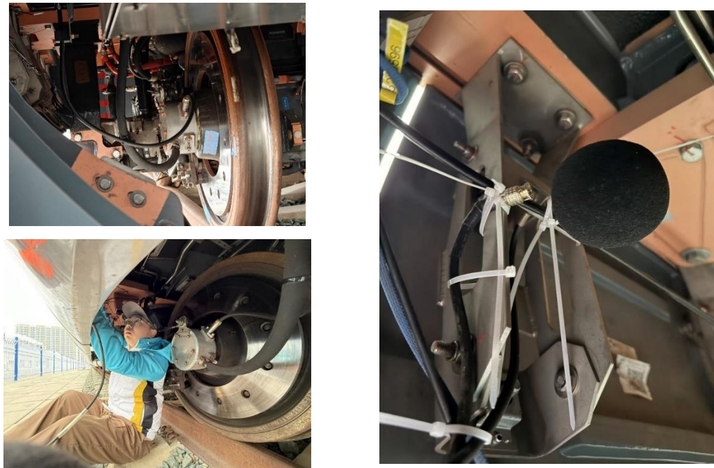
Fig 2.115 Layout of microphone sensors in the wheel-rail near-field
