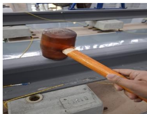
Fig 2.60 Experimental setup for railway track monitoring, (a) the DAS interrogator, (b) the rail tracks, (c) the optical fiber installed on the track and (d) the hammer to generate vibrations in the track
