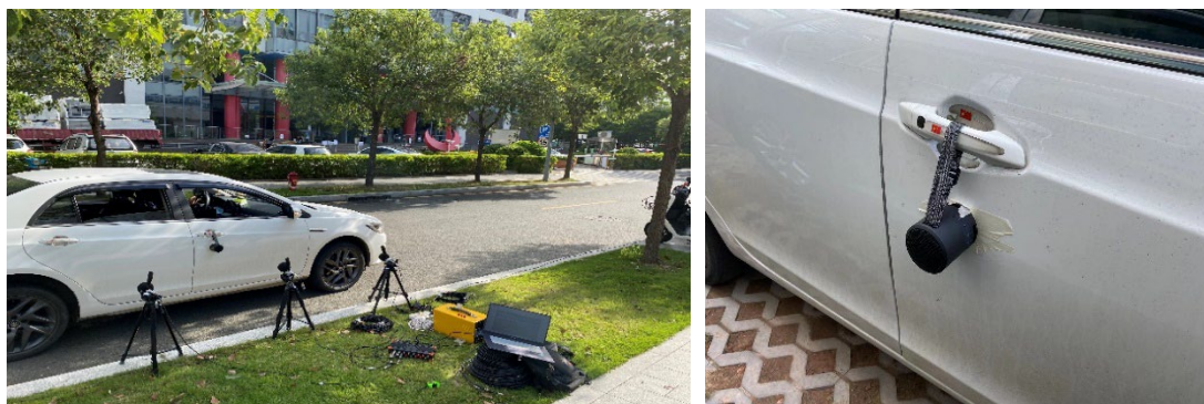
Fig. 2.14 Roadside test to simulate trackside test of bearing damage in train wheelset and loudspeaker fixing
