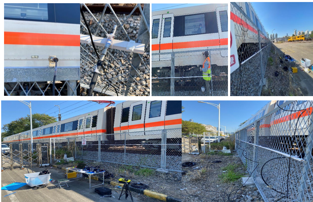
Fig. 2.16 Installation of trackside acoustic testing system for Shenzhen Metro
