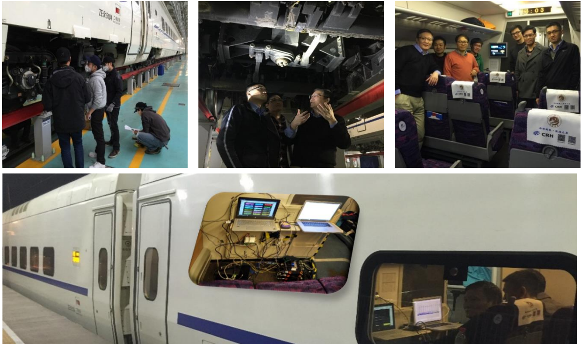
Figure 5-3 In-service comprehensive monitoring for assessment of high speed train dynamic behavior
