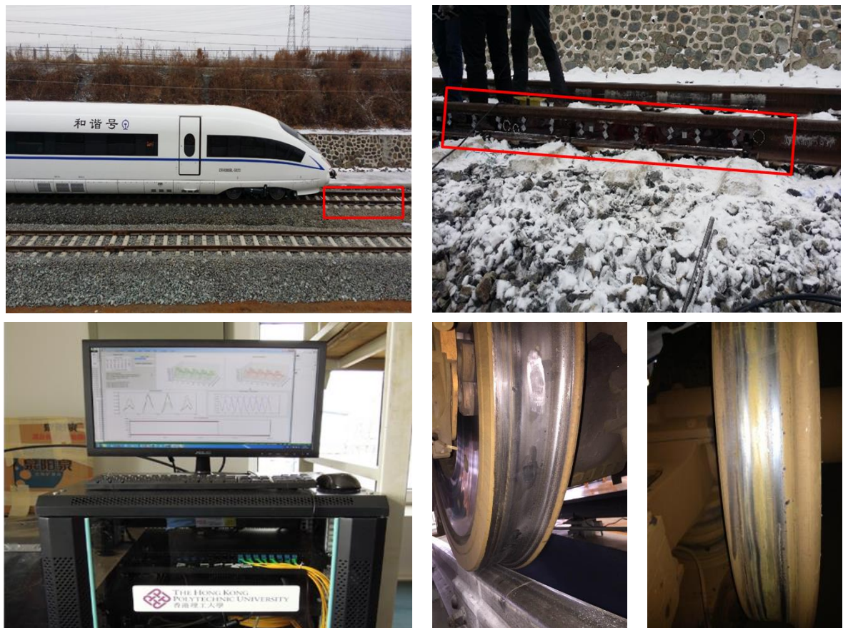
Figure 5-4 Application of monitoring system for wheel flat and wheel out-of-roundness identification
