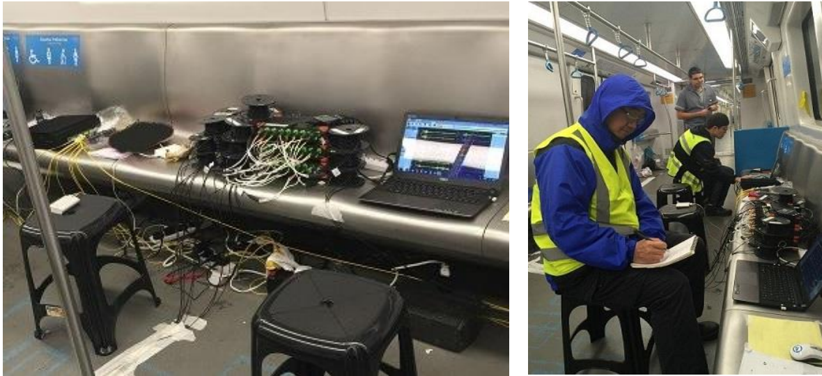
Figure 5-15 Analysis of data collected from the monitoring system on Brazil metro train
