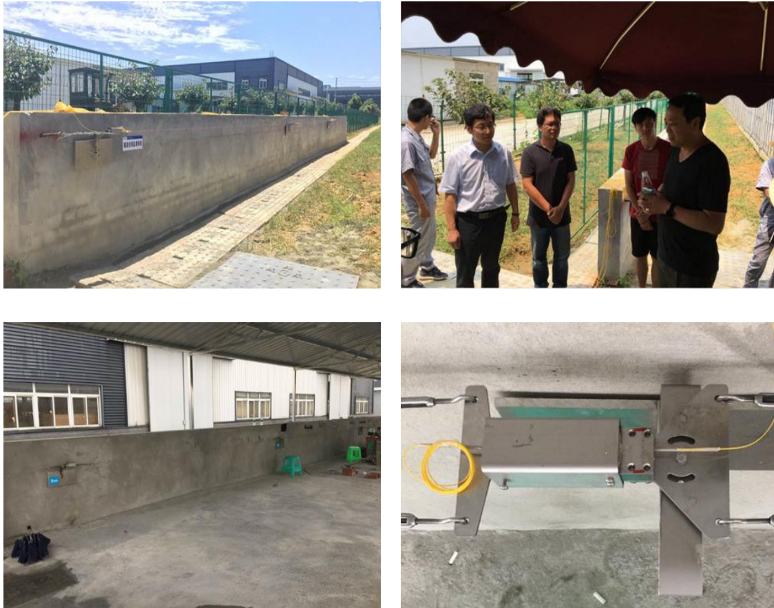
Figure 5-10 Full-scale experimental verification of the tunnel deformation monitoring system devised by CNERC-Rail
