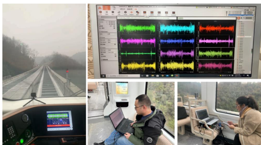
Figure 2. 6 On-line monitoring of the maglev train and guideway
