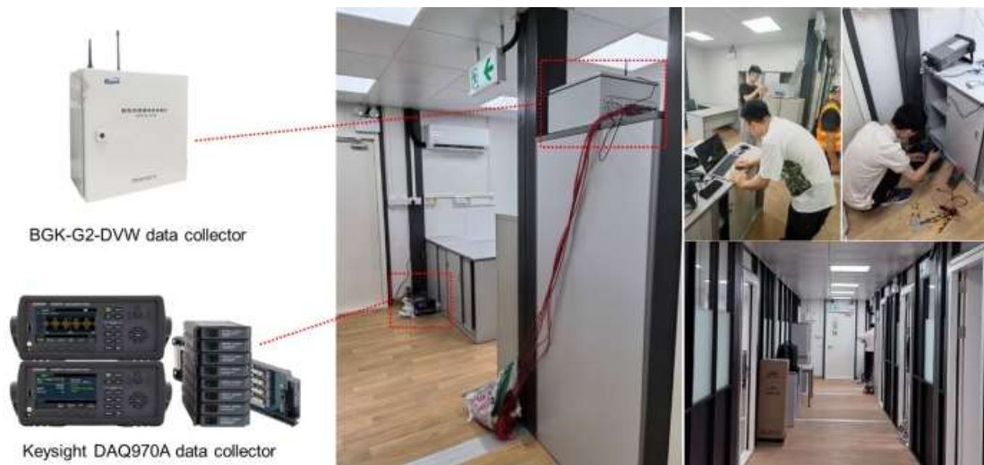
Fig. 2.26 Deployment and calibration of the on-site monitoring system in Yuen Long, Hong Kong
