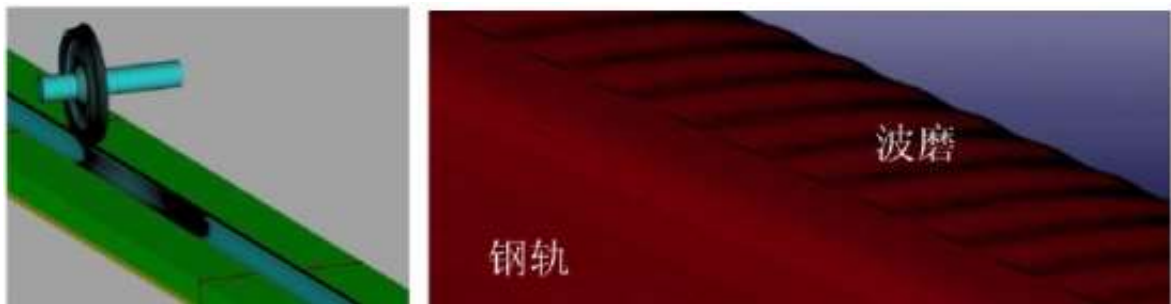
Fig. 2.18 Three-dimensional wheel-rail transient rolling contact modelling
