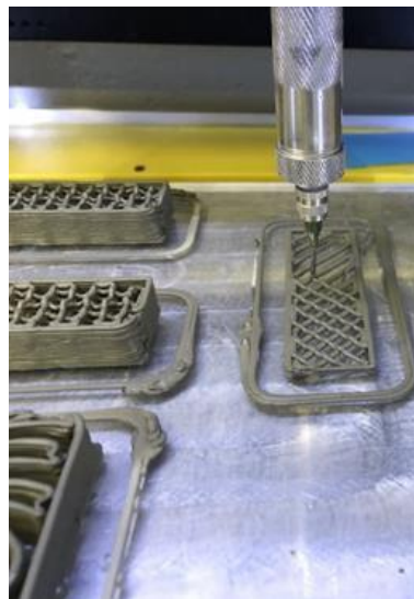
Figure 1. 3D printing of architected cement-based materials [Courtesy of M. Kosson and F. Sanchez, Vanderbilt University, 2021]
