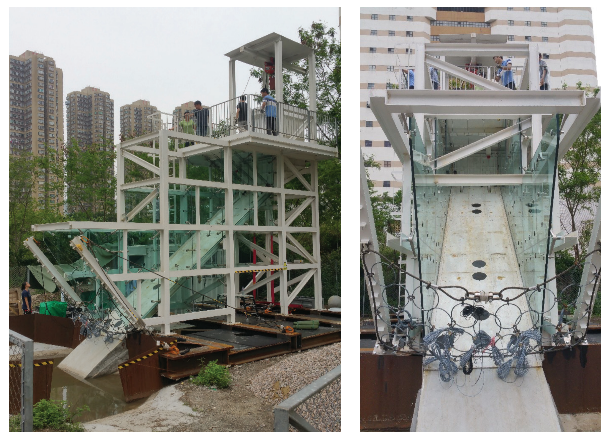
Plate 4: (a) An overall view of the facility (left) with a debris storage tank on the top, a flume, and a flexible barrier and (b) the front view of the flexible barrier with sensors and the flume (right)
