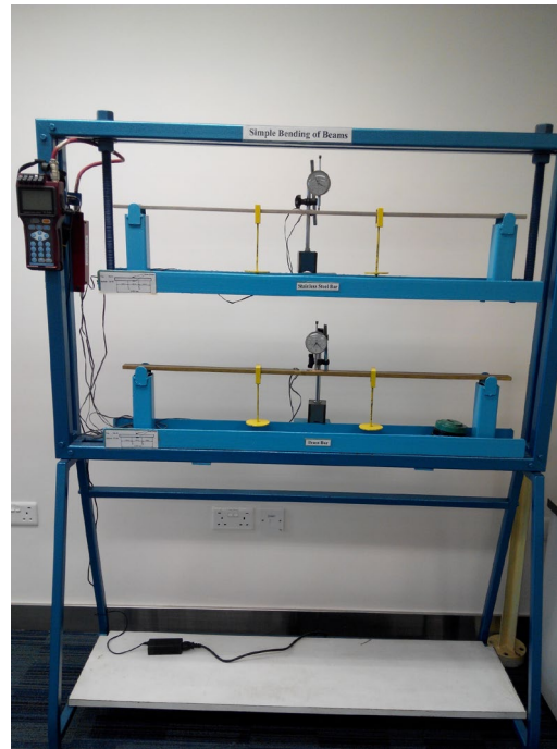
Simple bending of beams
