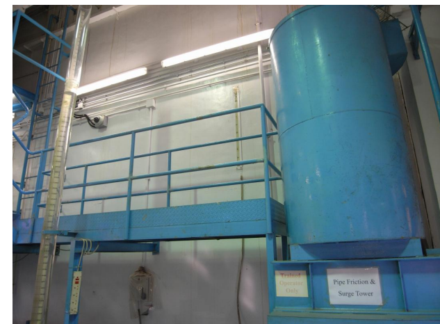
Pipe Friction and Surge Tower
