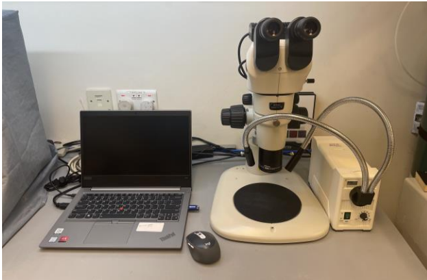
Nikon SMZ1270 Stereomicroscope with NIS Element BR Imaging Software
