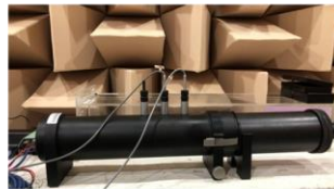
Primary path impulse response estimation
