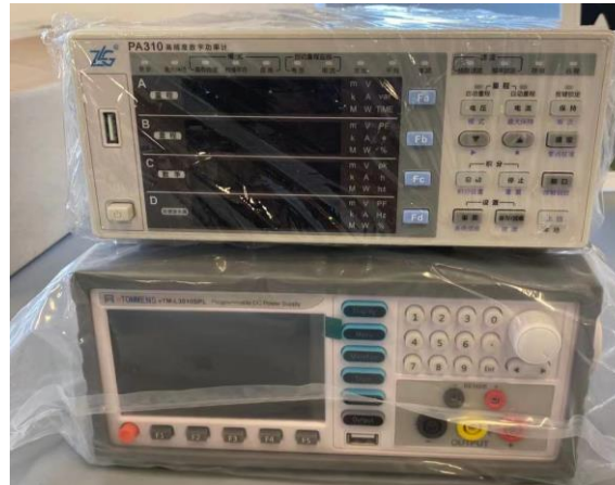
DC Power Supply & Power Meter
