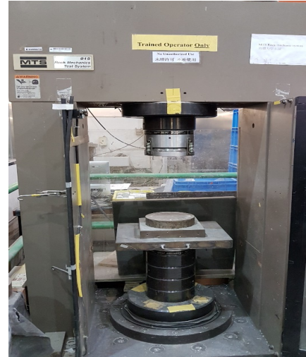
MTS 815 Test System
