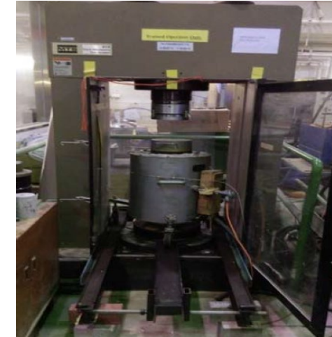
High-Temperature Furnace with MTS 815 Compression Test System
