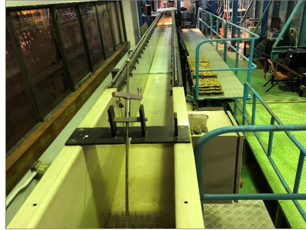
Open Channel (Tilting Flume)
