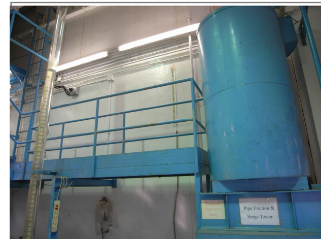
Pipe Friction and Surge Tower
