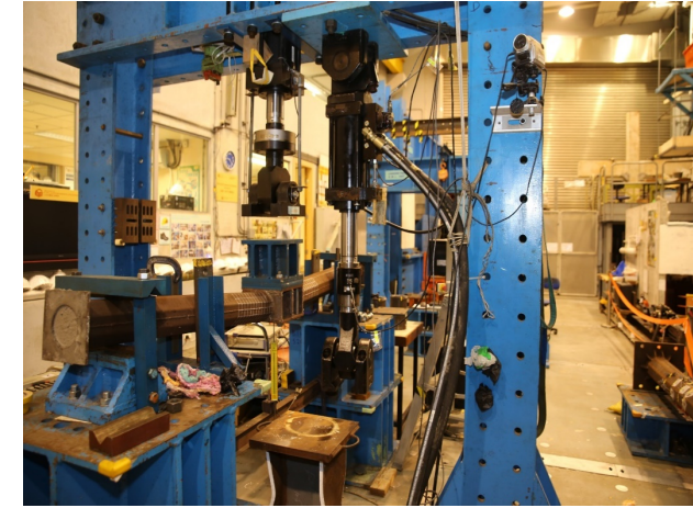
100 ton loading frame
