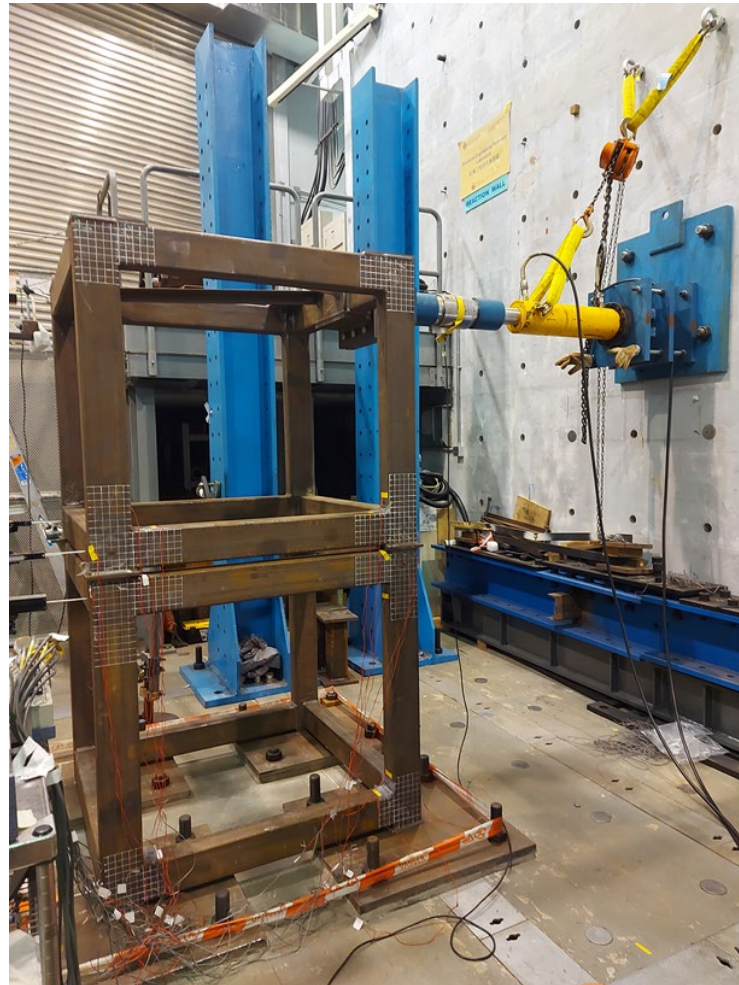
Steel frame joint test
