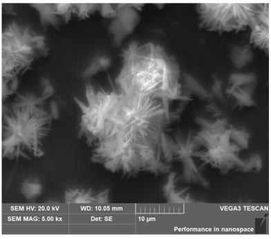
Micrograph acquired from Tescan Vega 3 XMU SEM showing Aragonite, the carbonation product of hydrated cement paste
