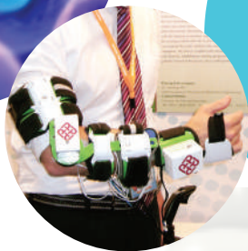
Rehabilitation sleeve: Robot & functional electrical stimulation (FES) hybrid system
