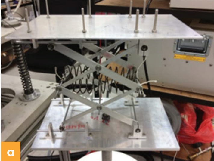
A prototype of the SLS platform: the prototype (a) and rollers in a horizontal track and bearings in rotational joints assembled in the system (b).
