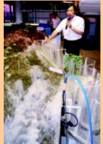
A miniature of the engineering structure of the Tsuen Wan drainage project has been built in the University's Hydraulics Laboratory. It took more than six months to construct this 1:20 physical model of the river, intake structure and device for simulating water flow during rainstorm warning. Dr Onyx Wai shows the model to the media in a press briefing.
