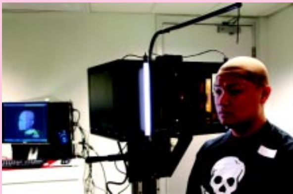
Mr Ball uses the 360 degree rotary, non-contact scanning machine (below), costing $800,000, to measure head sizes and facial features.
