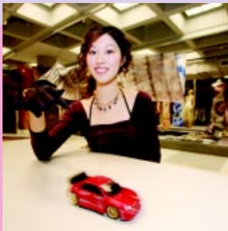
Sensing glove: Just by moving the fingers inside the glove, in which e-textile sensors are attached in the positions of finger joints, the demonstrator controls the motion of the racing car.
