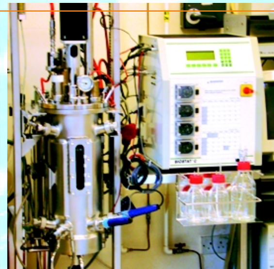
The computer-controlled fermentor plays a key role in the enzyme production process.
